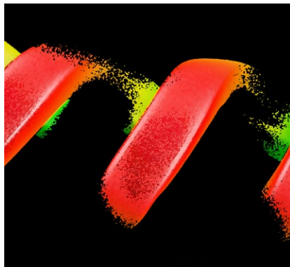
Scan data from a red laser sensor produces a more complete surface at the same exposure.
