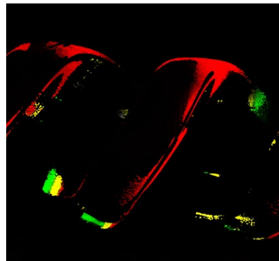
Scan data from a blue laser sensor produces significant data dropouts at the same exposure.
